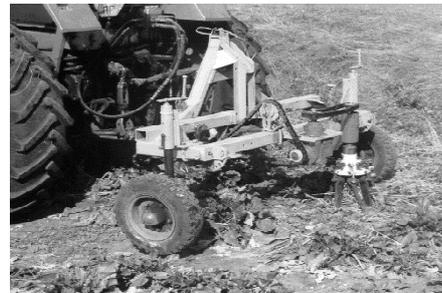
Fig. 2. **Sugar Beet Head Cleaner with a Vertical Cleaning Shaft**
